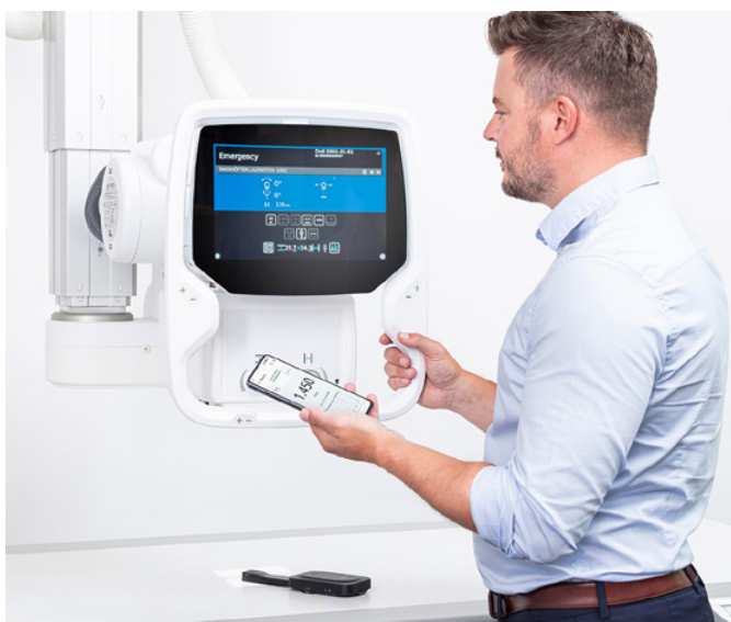
Figure 1. The App-powered Mako Display connects wirelessly to the Mako Meter.
